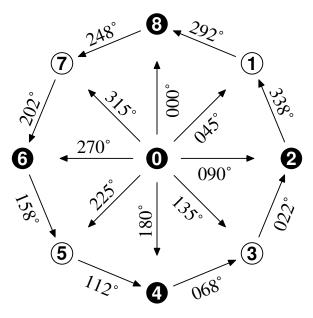
Bearings are shown in the diagram above. Interior angles are shown in the course diagrams below.
